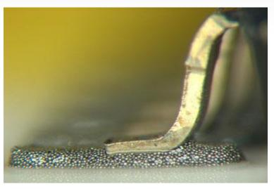
**QFP Lead in Paste, Prior to Reflow**
