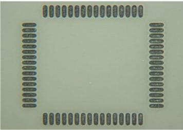
150um Thick Solder Paste Applied to the Ceramic Coupon
