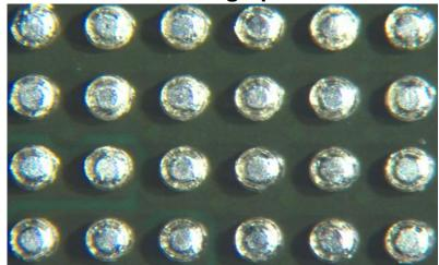
Flipped PBGA Where Applied Solder Completely Wet the Spheres
